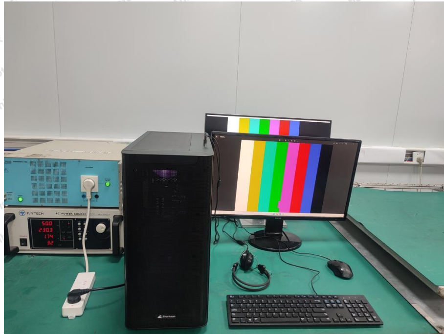
Photo of Harmonic Current And Flicker Test
