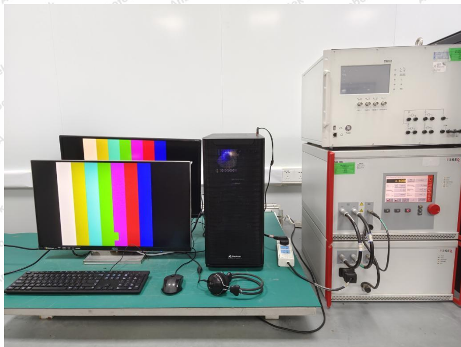
Photo of Electrical Fast Transient/Burst Immunity Test
