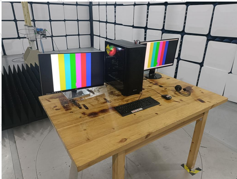
Photo of Radiated Emission Test (Above 1GHz)
