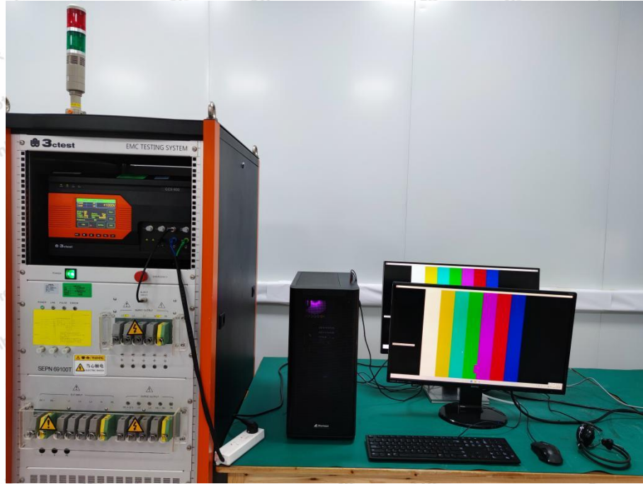
Photo of Surge Immunity Test
