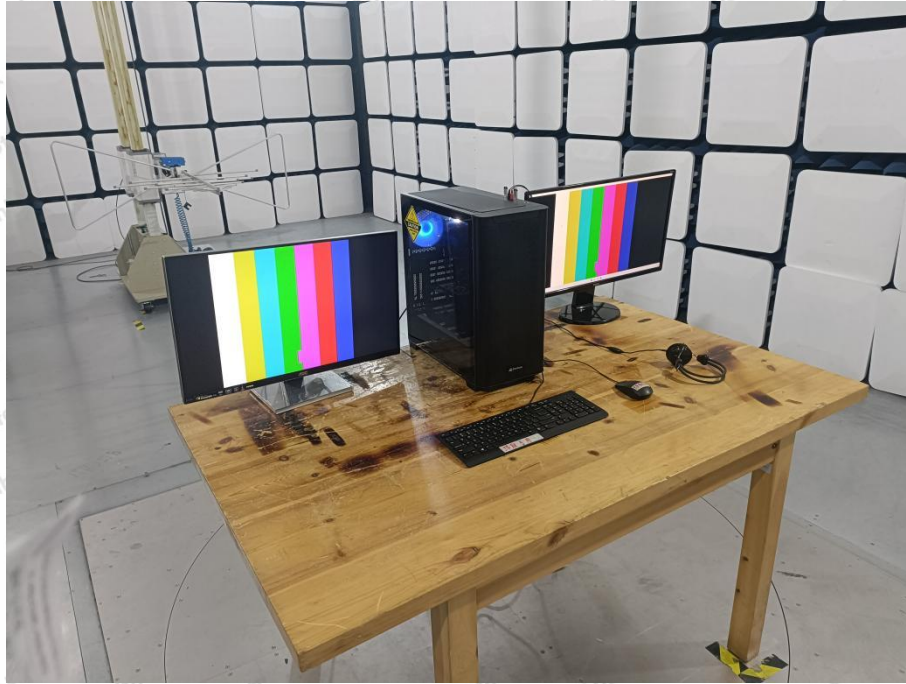
Photo of Radiated Emission Test (Below 1 GHz)
