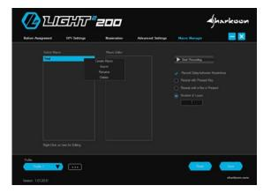
In the Macro Manager, macros with up to 50 key commands can be recorded, edited and deleted. Macros are independent of game profiles but can be used for any of these profiles after they have been recorded. Before a macro can be used, it must be assigned to a mouse button in the menu "Button Assignment". <u>Please note:</u> Depending on the keyboard and keyboard layout, certain keys are excluded from the macro recording.
