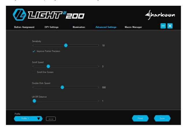
**Sensitivity:** With this option, the pointer speed can be adjusted. The higher the value, the faster the mouse pointer moves across the screen. In addition, the option "Improve Pointer Precision" can be activated. With this option, the faster the mouse is moved, the faster the mouse pointer moves.
