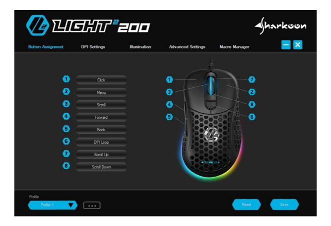
**Button Assignment:** The assignment of the eight buttons of the Light2 200 can be configured as desired. Individual keys can be designated with different commands, functions and macros.
