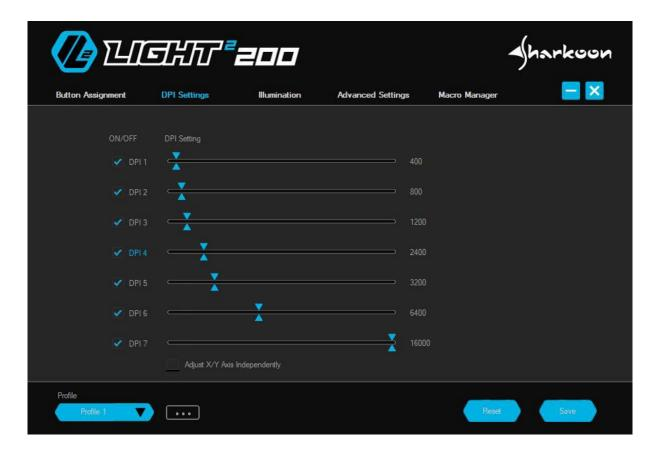
The seven DPI steps of the Light<sup>2</sup> 200 can be modified as desired. Each step can be assigned with a DPI value between 50 and 16,000. If required, the settings for the DPI values can be made separately for the X-axis and the Y-axis. The currently selected DPI step is highlighted in blue. DPI steps which are not needed can be deactivated.
